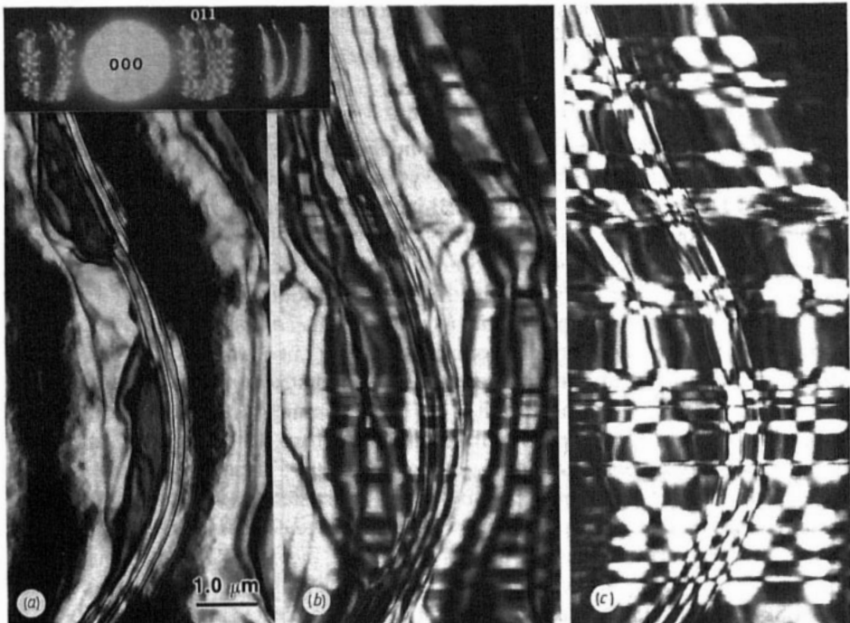
Figure 2. Imaging of the antiphase domains in \text{Bi}_2\text{Sr}_2\text{CaCu}_2\text{O}_8 . (a) bright-field imaged with a basic reflection (020), (b) and (c) bright-field and dark-field imaged with a superlattice reflection ( 01\bar{1} ). The curved band down the centres of the images is a group of four dislocation ribbons.
